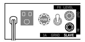
speaker, so any high frequency roll-off or other speaker coloration that you are used to hearing will not be present in this signal. Compensate for this at the mixing board or slave amplifier that you are using by rolling-off slightly the EQ Band that deals with the highest frequencies (5K and above), to simulate the sound of the amplifier's internal combo speaker. Lead sounds especially will require this high-frequency roll-off to avoid sounding thin and scratchy through the slave output.
